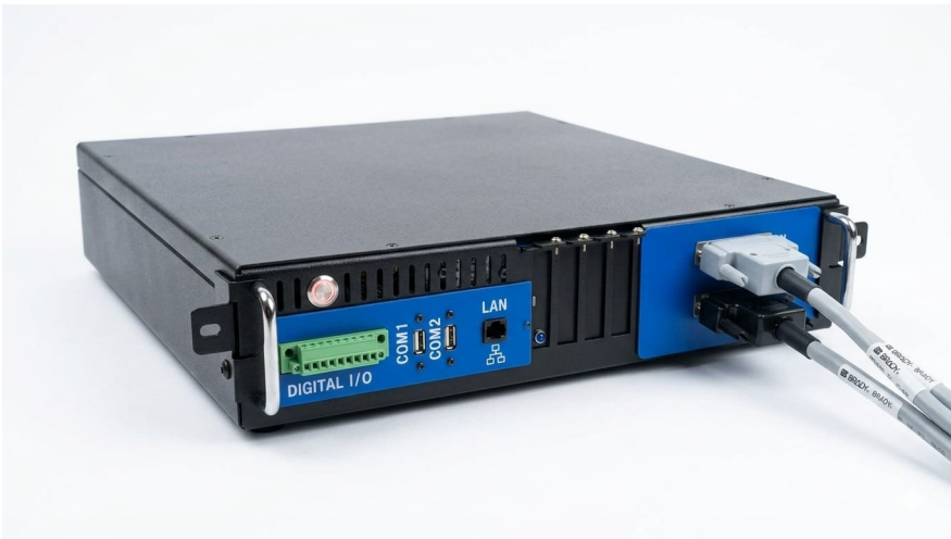
Figure 3.2 – OHM MATRIX with DB-50 cables connected
